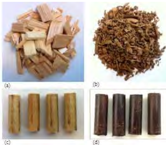
Figure 1- Appearance of raw material and pellets made in this study: (a) original Douglas fir woodchips, (b) SO 2 -steam treated and dried woodchips, (c) pellets made from untreated particles, (d) Pellets made from SO 2 -steam treated particles.
