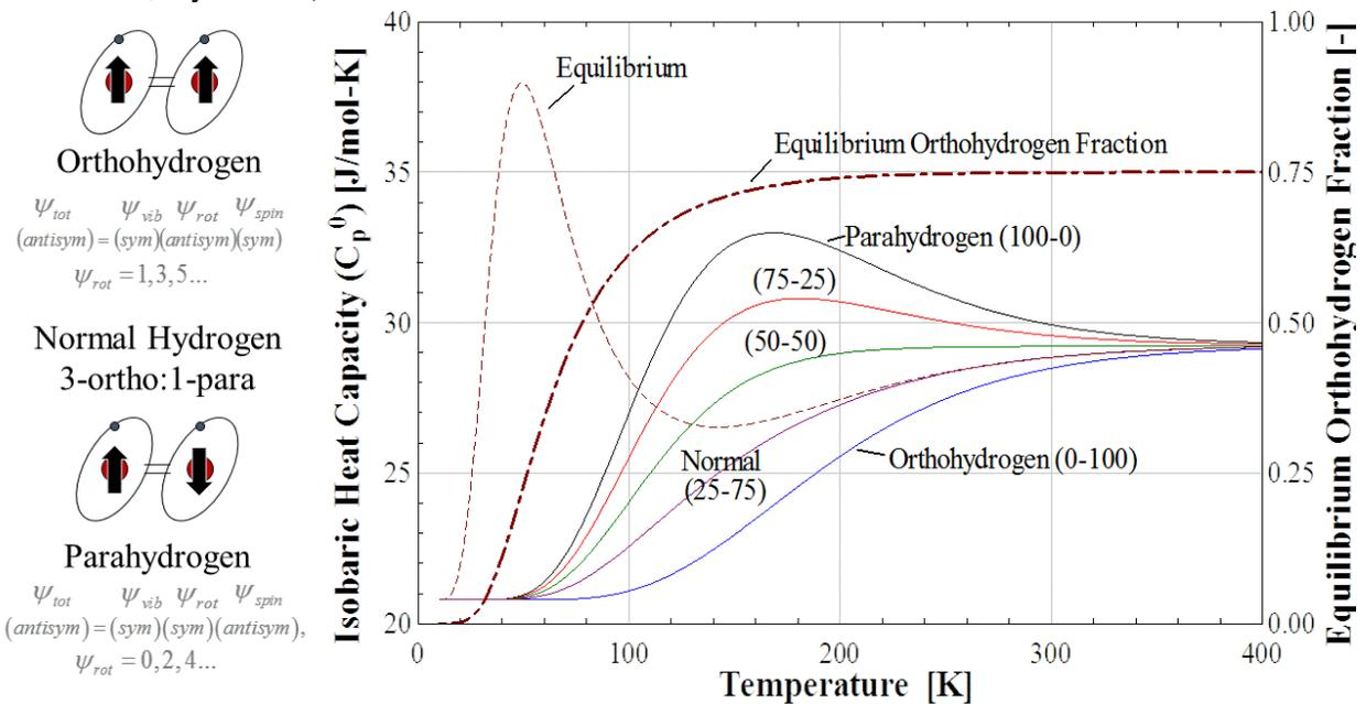
**Figure 2: Ortho-parahydrogen molecular wave function and ideal-gas isobaric heat capacities for various mixtures with the equilibrium orthohydrogen concentration.**
