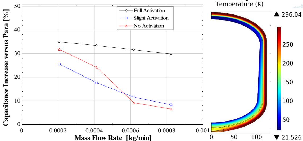
**Figure 3: (Left) Measured increase in cooling capacity during heating from 22-94 K in the presence of catalyst in the Cryocatalysis Hydrogen Experiment Facility (CHEF) (Bliesner *et al.* 2014). (Right) COMSOL multiphysics temperature model in a 3D-printed vapor-shielded tank with catalyzed para-ortho-hydrogen cooling (Adam & Leachman 2015).**
