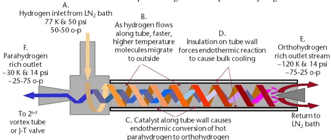
**Figure 1: Conceptual diagram of para-ortho-hydrogen conversion in a Ranque-Hilsch vortex tube.**
