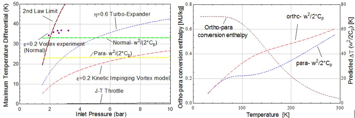
**Figure 4: (Left) Measured (pre-publication) and predicted refrigeration effects for hydrogen at 125 K. (Right) Ortho-parahydrogen conversion enthalpy and magnitude of temperature separation predicted by the  $w^2/2C_p$  model (Polihronov & Straatman 2012).**
